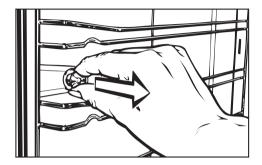
■ Pull on the fixing knob to release it.
